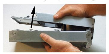
8. Separate the cooling unit section to access the blowers.
